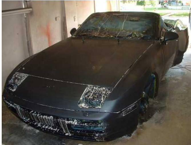
6 coats of paint and 3 coats of clear have been applied and the car is ready to be buffed
