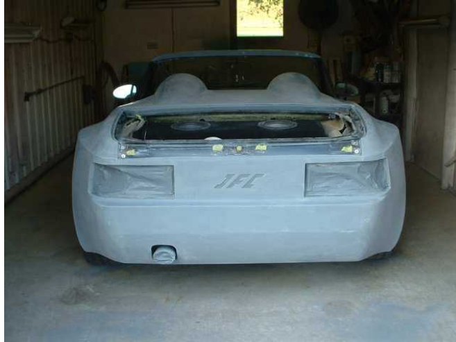
Prep work complete and primer applied
