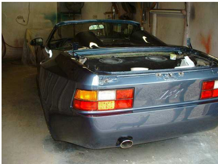
6 coats of paint and 3 coats of clear have been applied and the car is ready to be buffed
